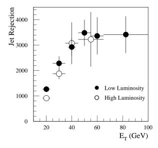
Figure 4.2: Expected ATLAS rejection factor for jets misidentified as photons as a function of  $E_{\text{jet}}^T$  after photon selection cuts for low and high luminosity [Atl99a].
