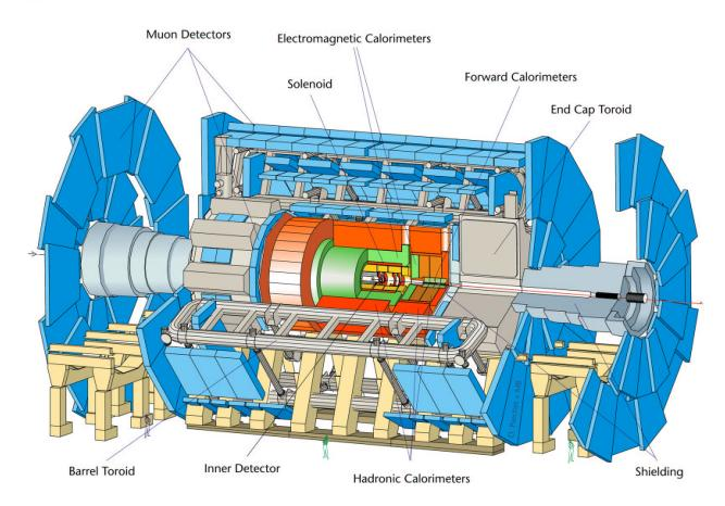
Figure 1.7: A cut-away view of the ATLAS detector is presented with the major sub-systems indicated [Atl99a, Fig. 1-i]. The outer radius of the detector is 11 m.
