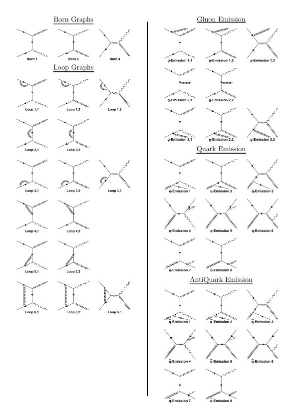
Figure 3.5: The Feynman graphs contributing to diboson production up to next-to-leading order in the strong coupling constant.
