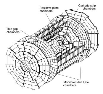
Figure 1.11: A three dimensional cut-away view of the ATLAS muon system is shown. The monitored drift tubes and cathode strip detectors provide high precision tracking measurements, while the resistive plate chambers and thin gap chambers are used primarily for fast triggering [Atl97b, Fig. 4-2]. The muon system has an outer radius of 11 m.
