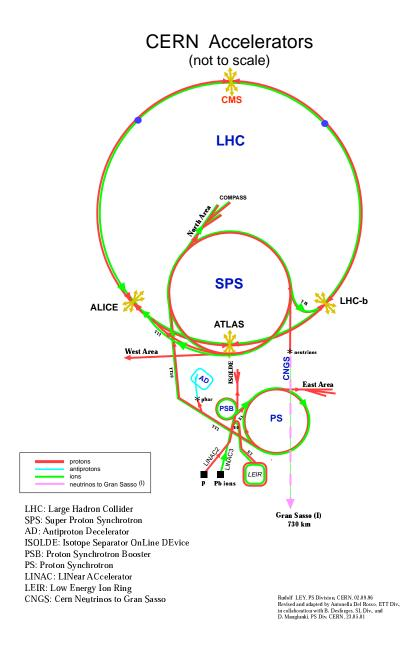
Figure 1.3: The accelerator complex at CERN is shown with the locations of the four LHC experiments ATLAS, CMS, LHCb, and ALICE indicated. The circumference of the LHC ring is  $26.7~\rm km$ .
