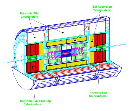
Figure 1.9: A three dimensional view of the ATLAS calorimeter system is presented [Atl99a, Fig. 1-iii]. The outer radius of the calorimetry system is 4.25 m.
